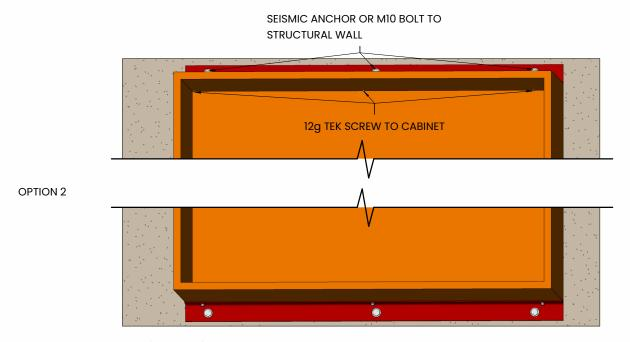
EQUAL ANGLE (50x2.5 EA) TO WIDTH OF CABINET AS PER DETAIL ON PAGE 16 FOR STRUCTURAL WALL OR DETAIL ON PAGE 17 FOR STUD WALL.
