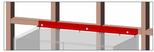
EQUAL ANGLE (50x2.5 EA) TO RUN THE ENTIRE LENGTH OF CABINET (WALL SHEETING OMITTED FOR CLARITY). 12g TEK SCREWS TO CABINET, 450 CTS MAX., MIN. QTY - 2.
