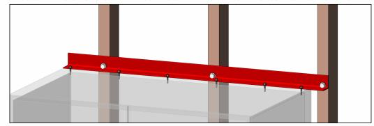
EQUAL ANGLE (50x2.5 EA) TO RUN THE ENTIRE LENGTH OF CABINET (WALL SHEETING OMITTED FOR CLARITY). 12g TEK SCREWS TO CABINET, 450 CTS MAX., MIN. QTY - 2.
