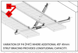
41mm STRUT WITH M10 FM1008, M10 BOLTS & FM1026 ANGLE BRACKETS. FM2324 BRACKET WITH 3-M10 BOLTS AND CHANNNEL NUTS JOIN 41mm AT 45°.
