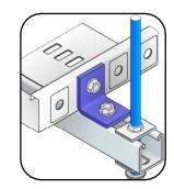
ALTERNATIVELY, FM1026 ANGLE **BRACKET WITH M10 DOME HEAD BOLTS THROUGH BOTH** TRAY AND 41mm CHANNEL
