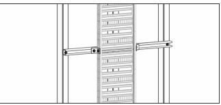
VARIATION TO ELECTRICAL RISER TO STUD WALL WHERE FM1026 BRACKETS AT 1000mm CENTRES ARE BOLTED 41mm STRUT WHICH IS BOLTED/SCREW-FIXED TO THE WALL STUDS. WALL LINING OMITTED FOR CLARITY.
