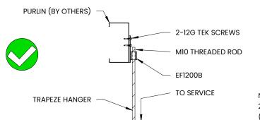
NOTE: FOR STAINLESS STEEL APPLICATIONS, 2-M10 NUTS REQUIRED, TYPICAL. (ABOVE AND BELOW EF1200B)
