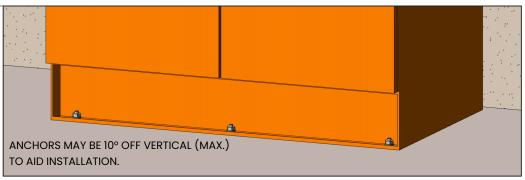
M10 SEISMIC ANCHORS TO CABINET BASE, WHERE PROVISION IS PROVIDED & MANUFACTURERS INSTALLATION INSTRUCTIONS ARE FOLLOWED. QTY TO SUIT, 900 CTS MAX., QTY - 2 MIN.
