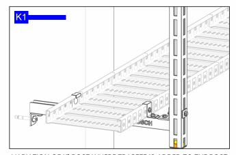
VARIATION OF K1 POST WHERE TRAPEZE IS ADDED TO THE POST WITH AN FM1026 ANGLE BRACKET AND M10 NUT AND BOLT. THIS ALLOWS POST TO CLEAR NEARBY OBSTICALS, OR TO FIX TO THE SOFFIT APPRIATELY.
