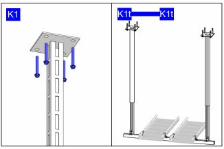
FIX 4- HILTI M10x90 HUS-H OR HILTI M10x90 HST3 OR M10x90 ICCONS FM753 OR APPROVED **EQUIVALENT. ALL INSTALLED IN ACCORDANCE WITH** MANUFACTURERS SPEC. 80mm MIN. EDGE DISTANCE.
