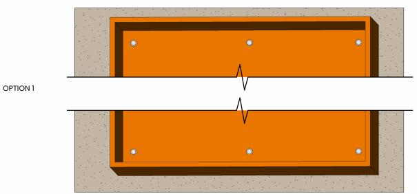
MIO BOLTS OR SEISMIC ANCHORS TO STRUCTURAL WALL (EXCLUDES STUD WALL). QTY TO SUIT, 900MM CTS MAX., QTY - 4 MIN.
