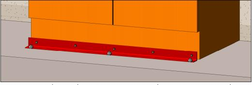
EQUAL ANGLE (50x2.5 EA) TO ENTIRE WIDTH OF CABINET. (OPTION - SIMILAR TO 2 SIDES) M10 SEISMIC ANCHORS TO EA. QTY TO SUIT, 900 CTS MAX., QTY - 2 MIN. 12g TEK SCREWS TO CABINET. QTY TO SUIT, 450 CTS MAX., QTY -3 MIN.
