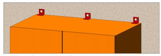
EQUAL ANGLE (50x2.5 EA) 50mm LONG (TYPICAL). MIO BOLT OR SEISMIC ANCHOR TO STRUCTURE, 900 CTS MAX., MIN. QTY - 2. 12g TEK SCREWS TO CABINET, 450 CTS MAX., MIN. QTY - 2.
