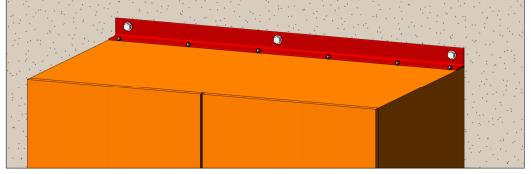
EQUAL ANGLE (50x2.5 EA) TO WIDTH OF CABINET. M10 BOLT OR SEISMIC ANCHOR TO STRUCTURE, 900 CTS MAX., MIN. QTY - 2. 12g TEK SCREWS TO CABINET, 450 CTS MAX., MIN. QTY - 2.
