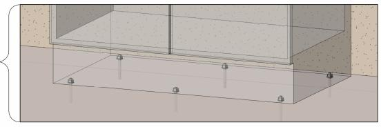
MIO SEISMIC ANCHORS TO CABINET BASE, PROVIDED THERE IS ACCESS AND THE MANUFACTURERS INSTALLATION INSTRUCTIONS ARE FOLLOWED. - NO FURTHER FIXING REQUIRED (INCLUDING TOP)
