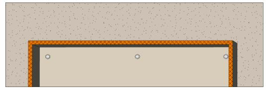
M10 BOLTS OR SEISMIC ANCHORS AT HIGH LEVEL. QUANTITY TO SUIT. 900 CTS MAX., MIN QTY - 2. (PROVIDED PROVISION IS MADE ACCORDING TO MANUFACUTERS INSTALLATION DIRECTION AND ACCESS IS AVAILABLE)
