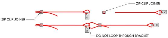
OPTION 2: ELIMINATE BRACKET, REMOVE FIXED LOOP WITH WIRE CUTTERS AND JOIN WITH ZIP CLIP JOINER
