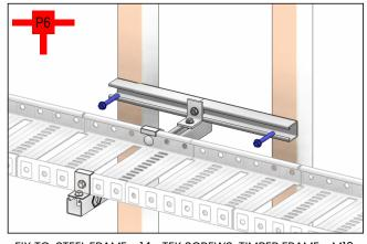
FIX TO: STEEL FRAME - 14g TEK SCREWS; TIMBER FRAME - M10 COACH BOLTS
