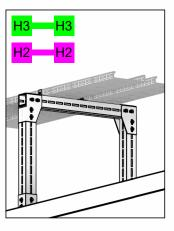
VARIATION TO H2 /H3 POST, WITH 2-SP80 / 100 -156 SHOE BRACKETS EACH WITH 8-SPBOLT-M12S. FIX TRAY TO HURDLE WITH TYPICAL HOLD-DOWN BRACKETS.
