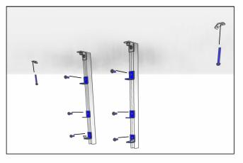
FIX FM1026 ANGLE BRACKETS TO SOFFIT WITH HILTI M10x90 HUS-H OR HILTI M10x90 HST3 OR M10x90 ICCONS FM753 OR APPROVED EQUIVALENT. ALL INSTALLED IN ACCORDANCE WITH MANUFACTURERS SPEC. 80mm MIN. EDGE DISTANCE.
