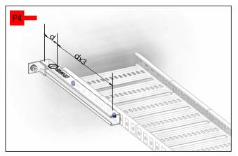
WHEN P4 IS PARALLEL TO TRAY, FIX WITH TWO M10 DOME HEAD BOLTS THROUGH DRILLED HOLES. ENSURE DISTANCE BETWEEN FIXINGS IS 3x DISTANCE FROM WALL U.N.O.
