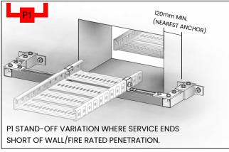
FM2346 BRACKET TO WALL WITH 2-M12 SEISMIC RATED ANCHORS AND 2-M12 BOLTS AND FM1008 TO SHORT PIECE OF 41mm STRUT.
