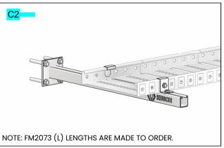
FIX FM2073 WELDED 41mm STRUT WITH HILTI M10x90 HUS-H OR HILTI M10x90 HST3 OR M10x90 ICCONS FM753 OR APPROVED EQUIVALENT. ALL INSTALLED IN ACCORDANCE WITH MANUFACTURERS SPEC. 80mm MIN. EDGE DISTANCE. FIXED WITH HOLD DOWN BRACKETS AND M10 BOLTS AND FM1008.
