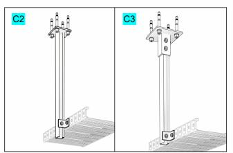
VARIATION OF WELDED **BASEPLATE 41mm STRUT** FIXED TO SOFFIT OR FLOOR WITH FM1026 ANGLE BRACKET AND M10 BOLTS TO TRAY
