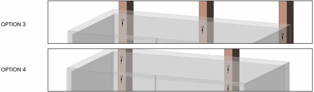
FIXING DIRECTLY THROUGH CABINET (WALL SHEETING OMITTED FOR CLARITY). STUDS AT 450 CTS - SINGLE ROW OF MIO COACH BOLTS (TIMBER STUDS)/12g TEK SCREWS (STEEL STUDS) QTY - 2 Min. STUDS AT 600 CTS - DOUBLE ROW OF M10 COACH BOLTS (TIMBER STUDS)/12g TEK SCREWS (STEEL STUDS) QTY - 4 MIN.
