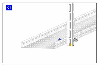
FIX TRAY TO POST WITH MIO DOME-HEAD BOLT AND STRUT WASHER THROUGH. ALTERNATIVLY, SP50-1068 (90°) BRACKET TO BOTH TRAY AND POST.
