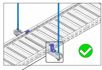
CABLE TRAY MUST BE INSTALLED WITH HOLD-DOWN BRACKETS AT EACH TRAPEZE HANGER
