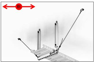
TYPICAL 2-WAY CABLE KIT TO TYPICAL TRAPEZE, SHOWN WITH ROD STIFFENERS FITTED. ALL TWO-WAY CABLE BRACES TO BE INSTALLED AT 90° TO DIRECTION OF SERVICE.
