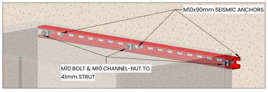
41mm STRUT TO WIDTH OF CABINET. M10 BOLT OR SEISMIC ANCHOR TO STRUCTURE, 900 CTS MAX., MIN. QTY - 2. M10 BOLTS & CHANNEL-NUTS TO CABINET, 450 CTS MAX., MIN. QTY - 2.
