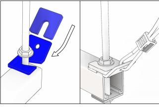
CABLE KIT BRACKET 'HOOKS' ONTO THREADED ROD. FIT SLOTTED SQUARE WASHER **OVER THE CABLE BRACKET** WITH EVERY KIT, IN THE ORIENTATION SHOWN.
