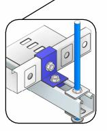
CABLE TRAY HOLD-DOWN BRACKETS WITH M10 NUT/BOLT TO BOTH CABLE TRAY AND 41mm STRUT TRAPEZE. TYPICALLY, DOME HEAD BOLTS TO TRAY ARE TO PREVENT BOLT HEAD TEARING CABLES AS THEY ARE PULLED.
