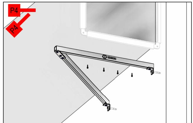
FIX TO: CONCRETE / CORE-FILLED BLOCK WALL WITH HILTI M10x90 HUS-H OR HILTI M10x90 HST3 OR M10x90 ICCONS FM753 OR APPROVED EQUIVALENT. (ALL ACCORDING TO MANUFACTURERS SPEC.)
