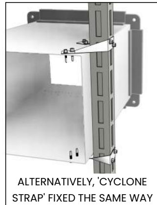
DRILL 12mm HOLES 100mm FROM EDGE OF DUCT & FIX 2-FM34HB10 WITH LOCKING NUT. THREADED ROD OR M10x120mm THROUGH SP50, LOCKED AS SHOWN WITH 2-LARGE FLAT WASHERS.
